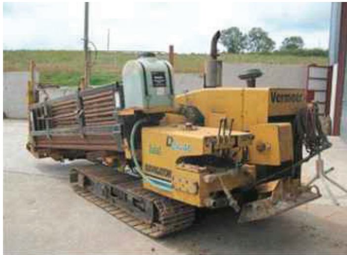
Typical Directional Drilling Rig
